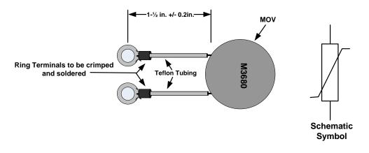
Mechanical and Electrical Diagram of the Site-Specific Solutions Model SSS-M3680 MOV Assembly
