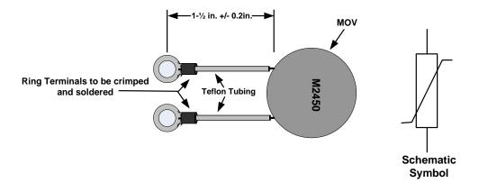
Mechanical and Electrical Diagram of the Site-Specific Solutions Model SSS-M2450 MOV Assembly
