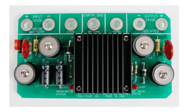
Photograph showing the SSS-12-24-ISO-48 Power Supply mounted to a standard AAR Terminal Block (not supplied)
